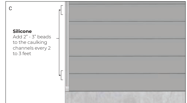
Silicone Add 2" - 3" beads to the caulking channels.
